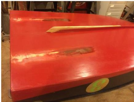
Granbery version: 12" keel removal, 1" added depth, trailing edge taper in both directions.
