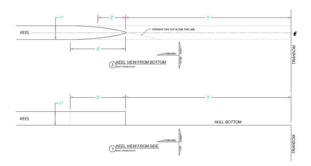
X = Total length of taper from trailing edge to final width. Must not exceed 4" +/- 1/2".
